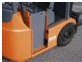
Low lift out battery extraction
